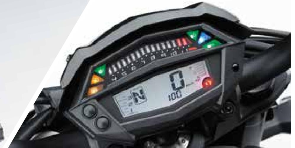
MULTI FUNCTION LCD INSTRUMENT PANEL
