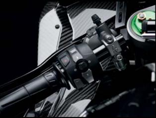
Compact new handle switch design allows all instrument functions to be controlled from the handles.
