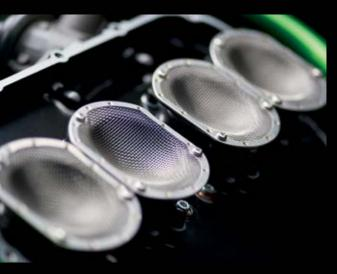
The top injectors spray fuel onto stainless steel nets positioned over the intake funnels. This has an ordering effect, creating a more uniform promotes fuel misting, which helps to cool the intake air and increases filling efficiency.
