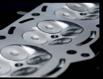
While the intake valves are stainless steel, the exhaust valves needed to be able to handle the supercharged engine's high-temperature exhaust gases. They are formed from two materials, friction-welded at the centre: inconel --an extremely heat-resistant alloy --is used for the head and lower half of the stem; heat-resistant steel is used for the upper half.
