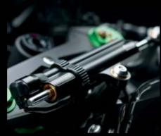
Kawasaki's electronic steering damper was jointly developed with Öhlins. Unlike a mechanical steering damper, the damping characteristics are changed electronically according to vehicle speed and the degree of acceleration or deceleration.
