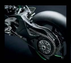
The Ninja H2R features Kawasaki's first singlesided swingarm. Having a single-sided swingarm were designed specifically for the Ninja H2R allows the exhaust silencer to be mounted closer to the bike centreline, ensuring a high bank angle for sporty cornering.
