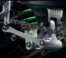
The bottom of the KYB fully adjustable mono rear shock is mounted via revised Uni-Trak linkage that offers excellent feedback regarding the rear tyre's grip condition to the rider. The new linkage, situated below the swingarm also mounts to the Swingarm Mounting Plate.
