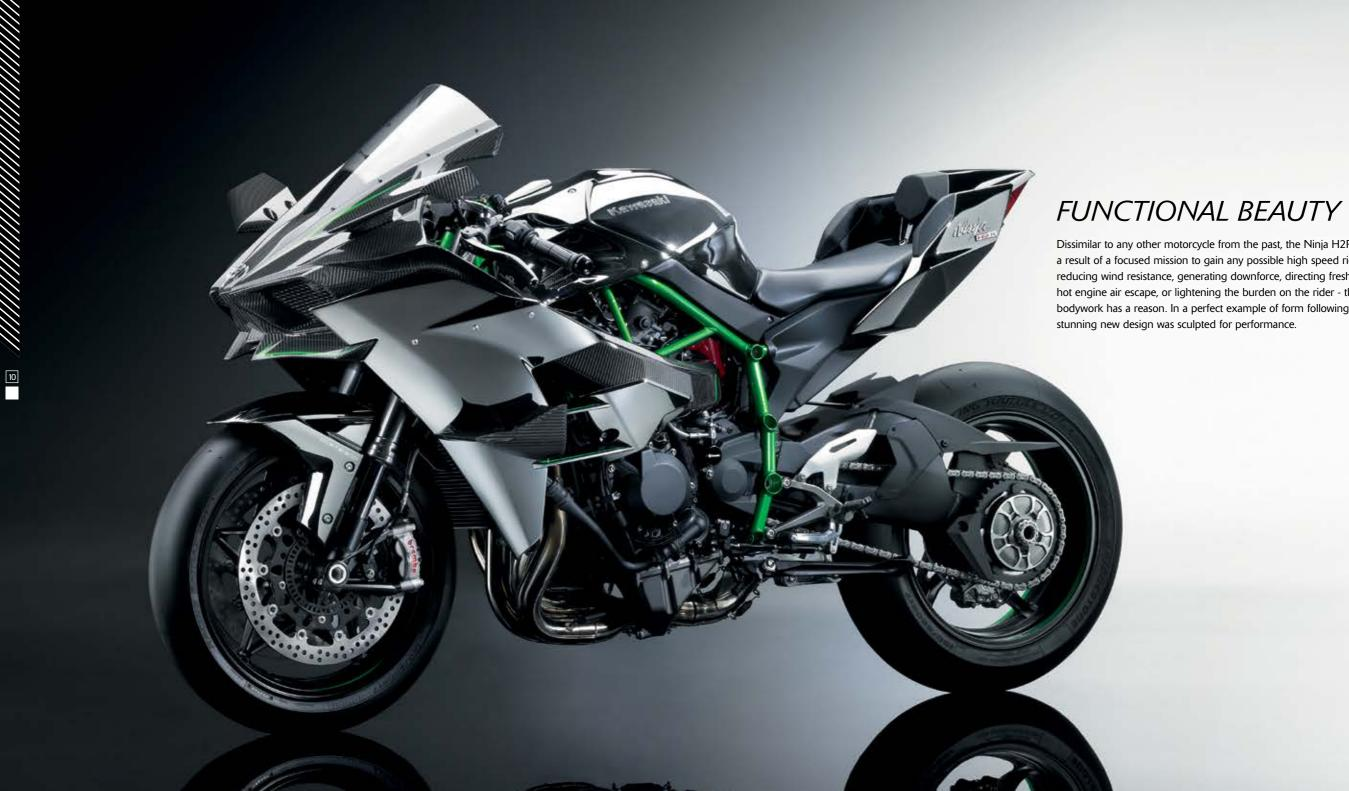
Dissimilar to any other motorcycle from the past, the Ninja H2R's exceptional form evolved as a result of a focused mission to gain any possible high speed riding advantage. Whether for reducing wind resistance, generating downforce, directing fresh air towards the engine, helping hot engine air escape, or lightening the burden on the rider - the shape of every piece of its bodywork has a reason. In a perfect example of form following function, the Ninja H2R's
