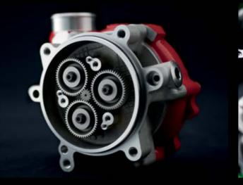
The Supercharger is driven by a planetary gear train, which runs off the crankshaft. Designing the gear train using technology from Kawasaki's Aerospace Company resulted in a very compact unit, with minimal power loss. fuel-air mixture as the fuel is sucked into the intake funnel. The net also
