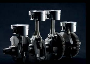
Cast pistons offer better strength than forged pistons for the very high temperatures generated by the high-performance engine. A unique casting process (similar to forging process) sees unnecessary material removed and hollows created to achieve the ideal thickness. This enables a light weight on par with forged pistons.
