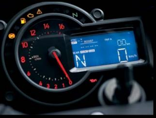
LCD screen uses a black/white reverse display. In addition to the digital speedometer and gear position indicator, display functions include: odometer, dual trip meters, current mileage, average mileage, fuel consumption, coolant temperature, boost indicator, boost temperature, stopwatch (lap timer), clock and the Economical Riding Indicator.
