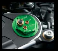
KYB AOS-II racing suspension makes its debut on an on-road bike. Based on the Air-Oil Separate cartridge fork developed for motocross racing, this is the industry's first use of this highperformance racing suspension on an on-road motorcycle.
