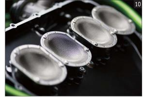
mixture as the fuel is sucked into the intake funnel. The net also promotes fuel misting, which helps to cool the intake air and increases filling efficiency. (Photo 10)
