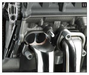
\* All-titanium exhaust system has a very simple design consisting of the header and collector pipes, a joint pipe, and a straightpipe megaphone-style silencer. (Photo 12)
