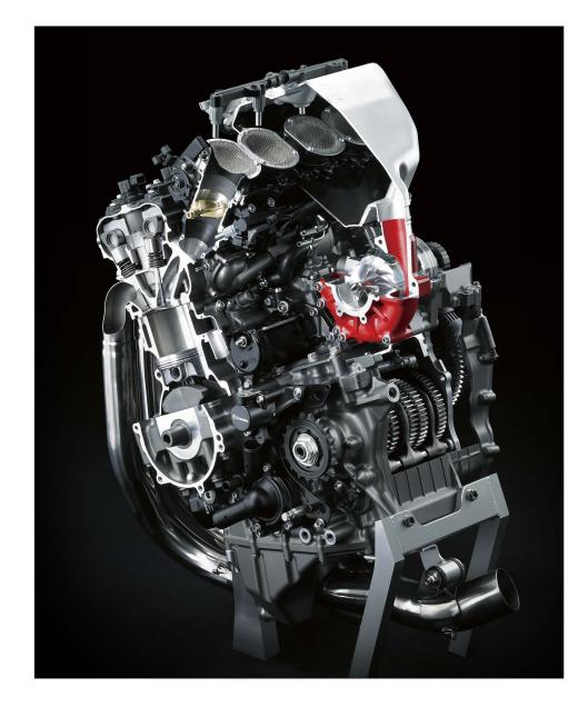
\* The supercharger the engineers designed is a centrifugal-type unit ideal for high-rpm performance—with a cast aluminium housing. (Photo 1)
