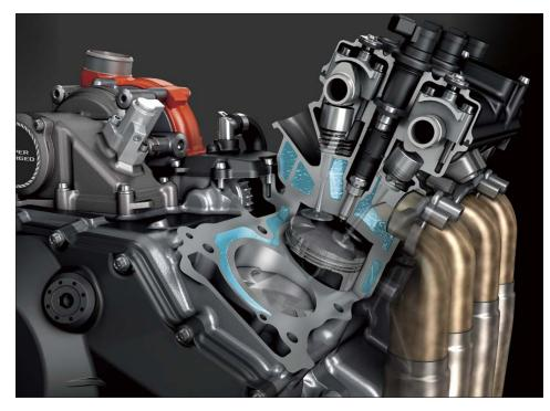
\* Water jacket extending between the twin exhaust ports of each cylinder, and large coolant passageways around the spark plug holes and the valve seat areas offer superior cooling. Spark plugs and valve seats, made of steel, have a greater tendency to retain heat than the aluminium cylinder head, so cooling them has a great effect.
