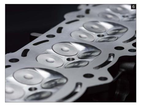
\* A dummy head is used during the cylinder honing process. The more precise circularity and cylindricity that result allow the use of low-tension piston rings, which helps reduce mechanical loss.
