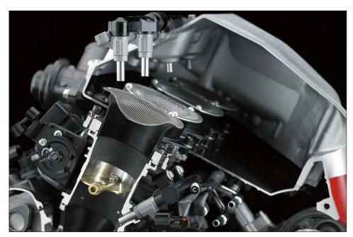
\* Intake chamber has a large volume (6 litres), and is ideally shaped for high efficiency and high engine output.
