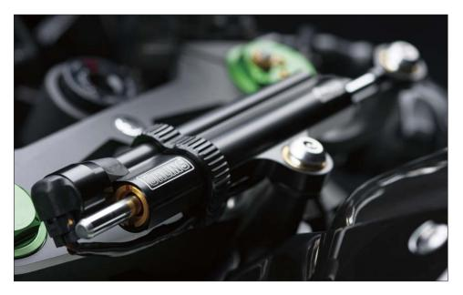
\* Kawasaki's electronic steering damper was jointly developed with Öhlins, one of the most popular and respected manufacturers of steering dampers.
