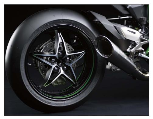
\* Star-pattern 5-spoke wheel design was selected based on analysis and testing to determine the optimum rigidity balance for ultra-high speed performance.
