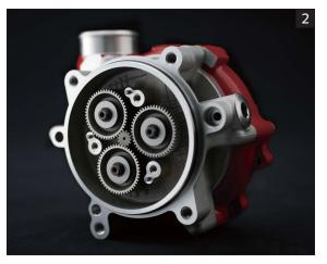
\* Gear train increases the impeller speed to 9.2x the crank speed (1.15x step gear x 8x planetary gear). This means that at maximum engine speed (approximately 14,000 min<sup>-1</sup>), the impeller shaft is spinning at almost 130,000 min<sup>-1</sup>. (Photo 3)
