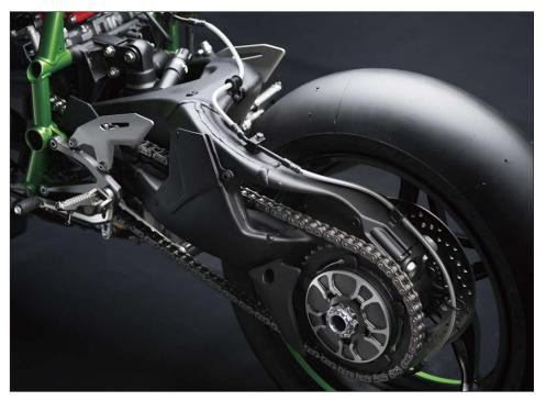
\* Having a single-sided swingarm allows the exhaust silencer to be mounted closer to the bike centreline, ensuring a high bank angle for sporty cornering.
