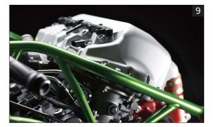
\* Inside the intake chamber, newly developed Kawasaki technology contributes to the engine's high performance. The top injectors spray fuel onto stainless steel nets positioned over the intake funnels (patent pending). This has an ordering effect, creating a more uniform fuel-air
