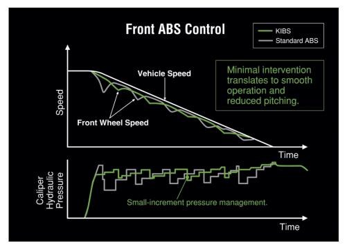
\* High-precision brake pressure control enables the system to avoid reduced brake performance due to excessive pressure drops, allows lever feel to be maintained when KIBS is active, and ensures ABS pulses feel smooth (not heavy).
