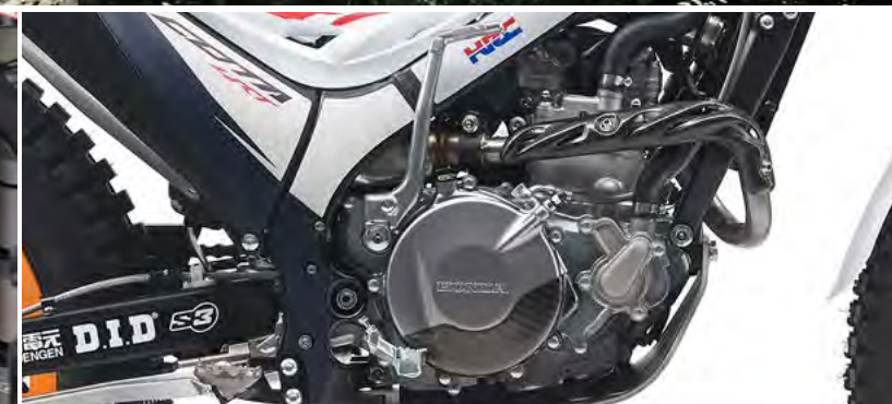
Carbon fiber clutch cover and exhaust elbow cover
