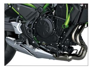
\* Revised duct joining the airbox and throttle bodies contributes to increased performance.
