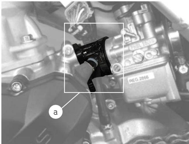
a) Reed valve, located between the carburettor and the engine.
