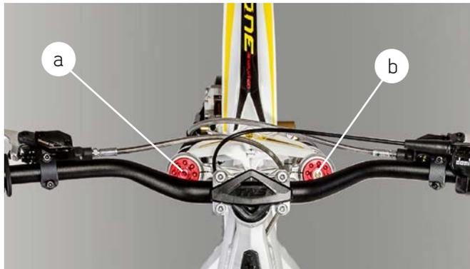
a) Spring preload; b) Adjusting the length
