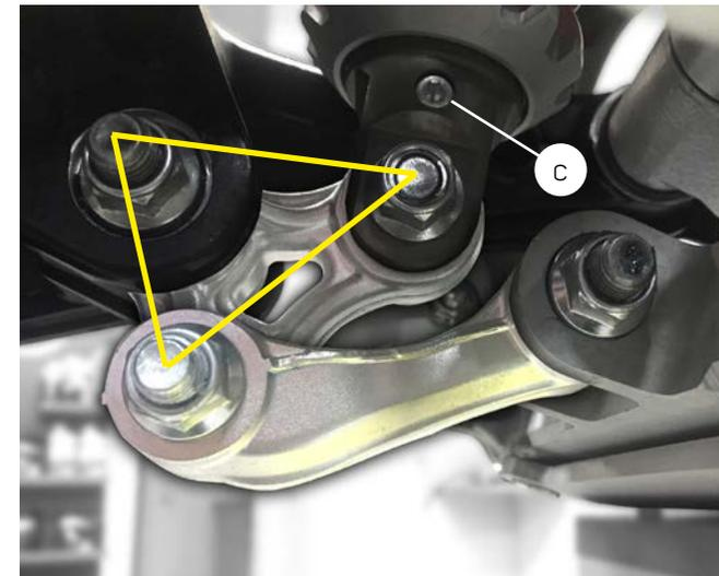
c) The hydraulic brake of the shock absorber can be adjusted using the screw located on the bottom.
