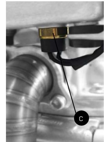
b) Temperature switch located at the bottom of the radiator.
