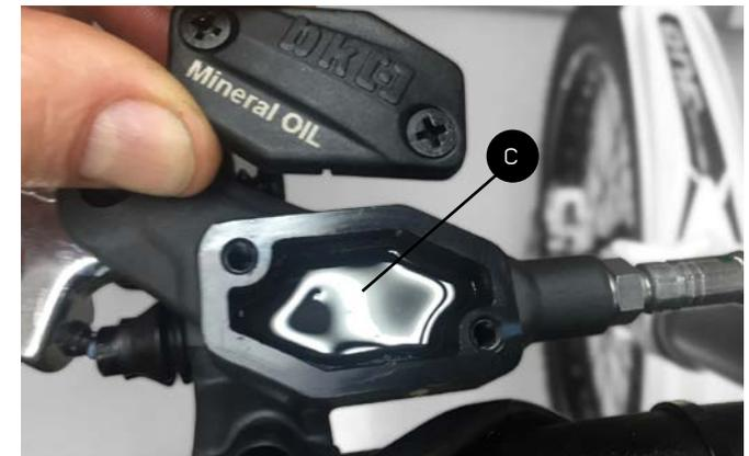
c) Clutch pump tank. Only mineral oil may be used, in order not to damage the o-rings
