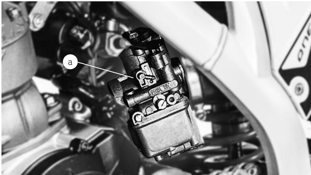
a) Carburettor. When handling the carburettor and adjacent parts there may be traces of fuel that need to be drained first.
