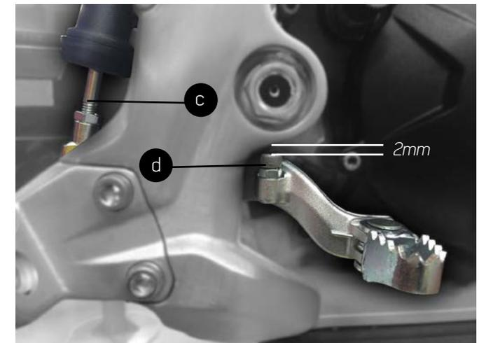
c) Tensioning rod rear brake pedal; (d) Screw for height adjustment of the brake pedal. For correct performance, you need to leave a small clearance gap.
