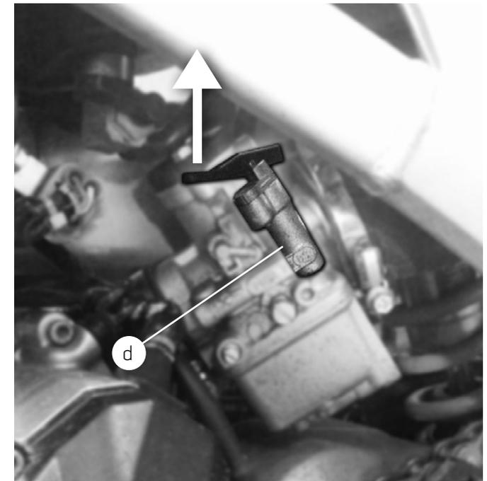
d) Choke, in the carburettor
