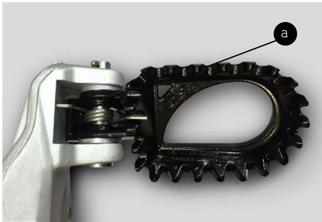
a) The footrests are adjustable, so that you can move them forwards or backwards by moving the washers 2.5mm to 5.00mm in either direction.
