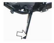
To use the main, depress it by foot and lift the rear of the motorcycle until the rear wheel is lift. To use the side, depress the end of it until it rotates to the Function of Controllers end and stops.
