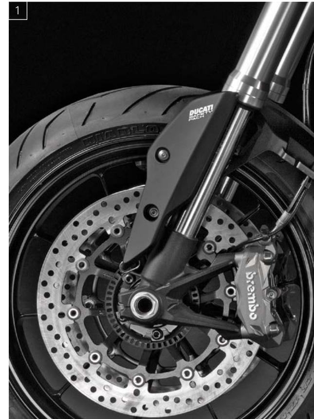
1. Pinza Brembo Monoblocco ad attacco radiale con ABS Bosch 9MP, parte integrante del Ducati Safety Pack (ABS+DTC) / Brembo monobloc radial callipers with Bosch 9MP ABS, an integral part of the Ducati Safety Pack (ABS+DTC)
