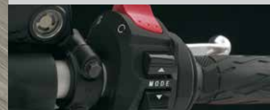
Suzuki Drive Mode Selector (S-DMS)
