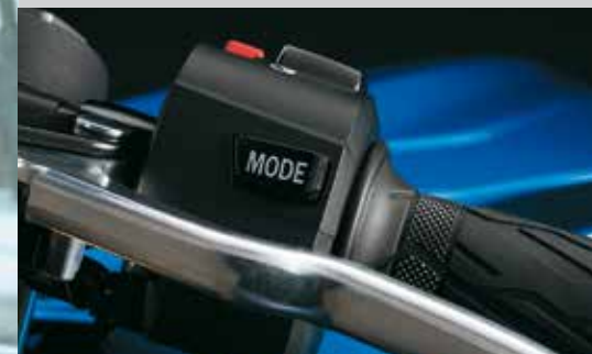
Suzuki Drive Mode Selector (S-DMS)
