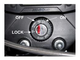
LOCK position — all electrical circuits are cut off and the engine will not start. The steering lock is actuated and the handlebar cannot turn. The key can be removed. To pass to lock position, the switch must be in OFF position and the pushed down and turned to the left. The handlebar must be turned all the way to the left.
