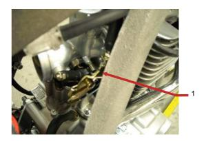
The idle sped is controlled by means of the mixture control screw (1). Turning the mixture control screw clockwise reduces the fuel quantity (lean mixture); turning counter-clockwise increases the fuel quantity (rich mixture).
