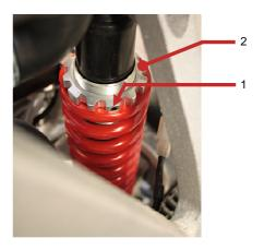
To adjust pre-charge, loose first the fixation screw (1). Turn adjusting nut (2) clockwise for more pre-charge or counter clockwise for less pre-charge.
