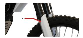
The dust protection gaskets (1) are to remove dust and coarse dirt particles from the fork tube. However, after some time, dirt may also get behind the dust protection gasket. If this dirt is not removed, the oil sealing rings located behind it may start to leak.
