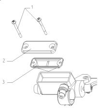
Loosen screws (1), remove cover (2) and membrane (3). Place hand brake cylinder in a horizontal position and fill the brake fluid reservoir up to the MAX mark with clean brake fluid DOT 4. Replace membrane, lid and tighten screws. Clear off spilled or overflowing brake fluid with water.
