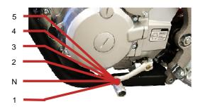
To shift properly, pull the clutch lever and close he throttle at the same time you operate gearshift lever. Lift the lever to up-shift and depress to downshift.
