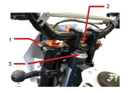
Check steering head bearings for play periodically. For check, place motorcycle on a stand so that the front wheel is off the ground. Try to move the fork forward and backward. For readjusting, loosen top nut (2) and the
