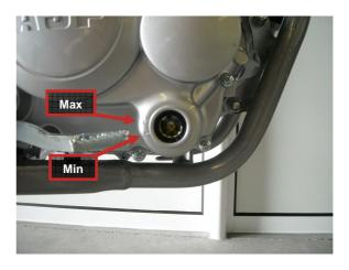
If oil level is below Min, oil must be refilled immediately. If you check that
