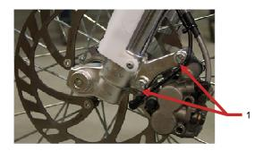
Clean the brake calliper and calliper support with compressed air. Check the sleeves of the guide bolts for damage and grease guide bolts if necessary. Mount both brake pads and then insert the clips the right way, to allow brake pads to jump off or lose, in order to avoid accidents.
