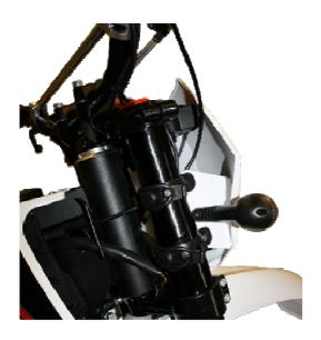
When placing a new lamp, do not touch the glass body of the lamp so it remains free from fat. Engage retaining clip and mount rubber cap and connector. Reinsert parking light lamp together with holder and fix the mask by means of the rubber bands.
