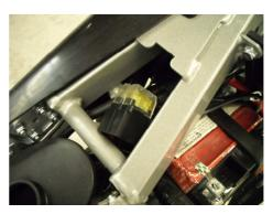
The fuse capacity is 20 Ampere, except for MX versions, which is 10 Ampere.
