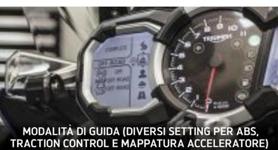
MODALITÀ DI GUIDA (DIVERSI SETTING PER ABS, TRACTION CONTROL E MAPPATURA ACCELERATORE)
