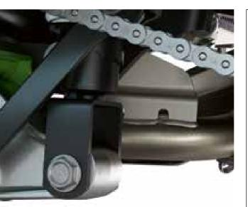
UNI TRAK REAR SUSPENSION FOR GREAT ROAD HOLDING ABILITY AND BUMP ABSORPTION
