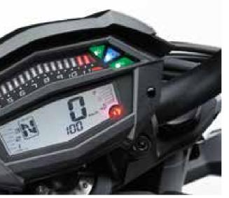
MULTI FUNCTION LCD INSTRUMENT PANEL
