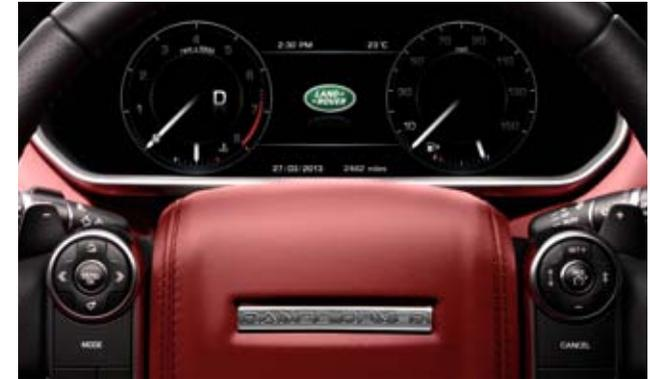
**Full Thin Film Transistor (TFT) Instrument Panel**
