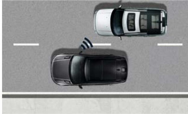
**Blind Spot Monitor with Closing Vehicle Sensing**
