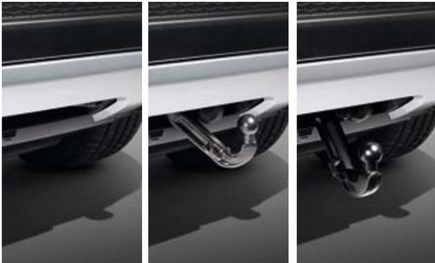
Electrically Deployable Tow Bar
