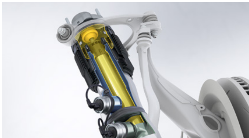
Adaptive air suspension with three-chamber technology
