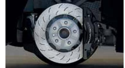
Black calipers standard on Grand Sport and available on Stingray and Z06<sup>7</sup> (Brembo<sup>®</sup> slotted brakes included with available Z51 Performance Package shown)
