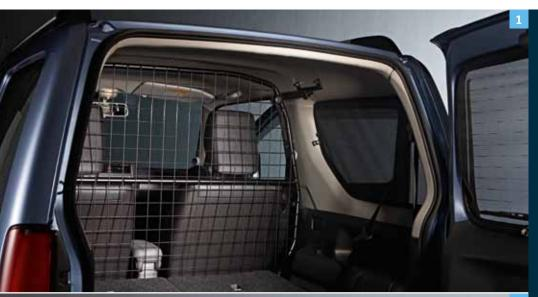
1 | Partition grid steel, easy to remove Part No. 00800-41268-GIT
