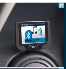
17 | Bluetooth®² system, Parrot MKi9200 additional options: Compatible with SD and SD-HC card. Sound equaliser with digital class-d 20W amplifier. TFT-Display (72 x 57 x 12mm). Displays CD covers or pictures. Includes Suzuki specific wiring harness.
