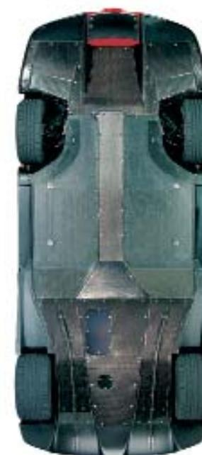
As the speed increases from low-medium to high-very high, the engineering ensures that the car takes on the optimal aerodynamic set-up (maximum downforce obtained with an optimal load distribution) by varying the rigidity on the basis of ground clearance. As the speed climbs even higher, this set-up is maintained by the combined action of the flexible mechanical components and by active control of the spoilers. This means that even if the intensity of
